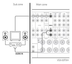
Different sources can be playing in two zones at the same time or, depending on your needs, the same source can also be used. The main and sub zones have independent power (the main zone power can be off while the sub zone is on) and the sub zone can be controlled by the remote or front panel controls. However, you may need to specify the volume settings in *ZONE Audio Setup* on page 72.
